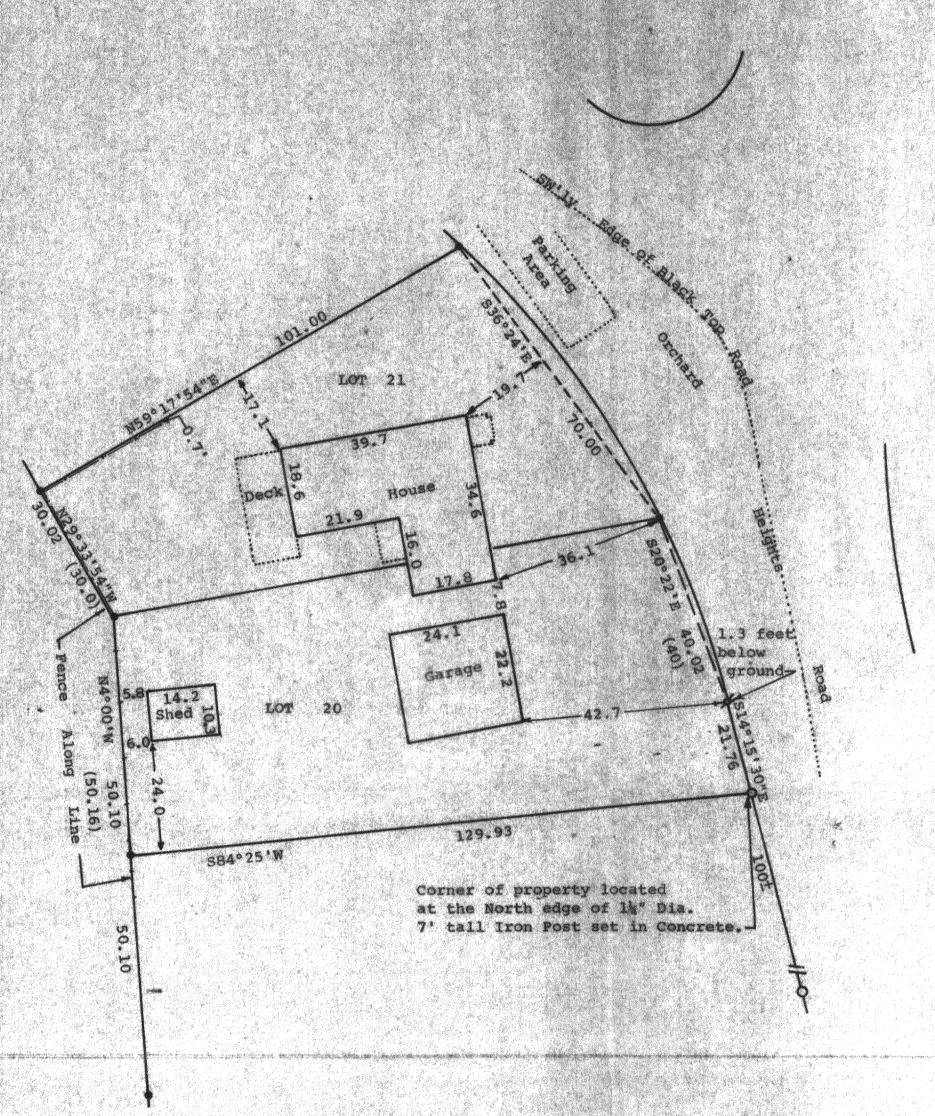
Scale -1" = 20"• = 5/8" Dia. Iron Rod Found  $p = \frac{1}{2}$ " Dia. Iron Rod Found O = 14" Dia. Iron Pipe Found (0.0) = Recorded Distance Bearings are referenced to the west line of Lot 20, Assumed bearing of N4°00'W.
